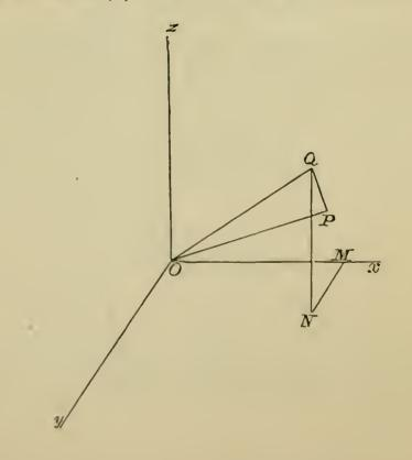
If, in the figure of that Article, QN be drawn parallel to the axis of z to meet the plane of xy in N, and NM drawn parallel to Oy to meet Ox in M, it follows that the projection of OQ on OP is equal to the sum of the projections of OM, MN and NQ on OP, that is, if  $\theta$  be the angle POQ, and l, m, n; l', m', n' be the direction-cosines of OP and OQrespectively,
